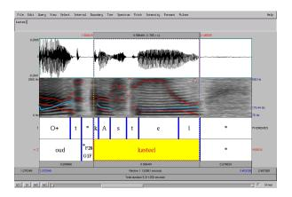
Formants (red dots) and Pitch (blue line) can be automatically determined and plotted into a spectrogram.
