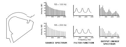
Sound enters the oral cavity (vocal tract) from below and is filtered by the resonances of the cavity
