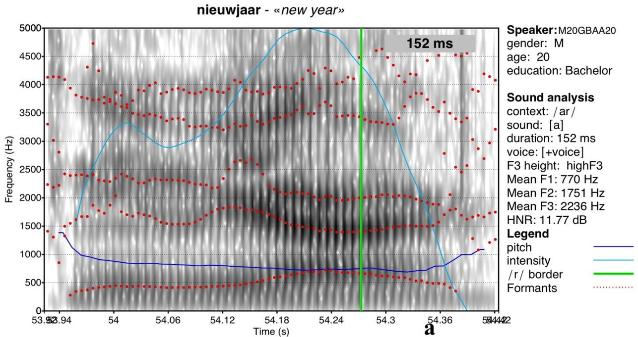
**Fig. 9.9.** Spectrograms of *nieuwjaar* ‘new year’ (speaker M20GBAA20) performed through Praat v. 5.3. On the right all the details that signal the sound as a vowel: a voiced sound with a high value of F<sub>3</sub> and a high value of the HNR. The correlations of F<sub>1</sub> and F<sub>2</sub> brought to the result of an [a]. F<sub>3</sub> height is labelled as ‘high’ that is above 2,000 Hz.
