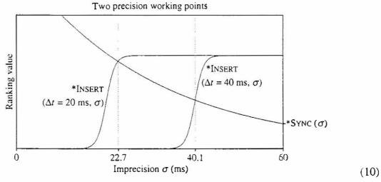
In this example, a timing difference of 20 or 40 ms leads to a working point of 22.7 or 40.1 ms, respectively. We can see all three local rankings in the figure.
