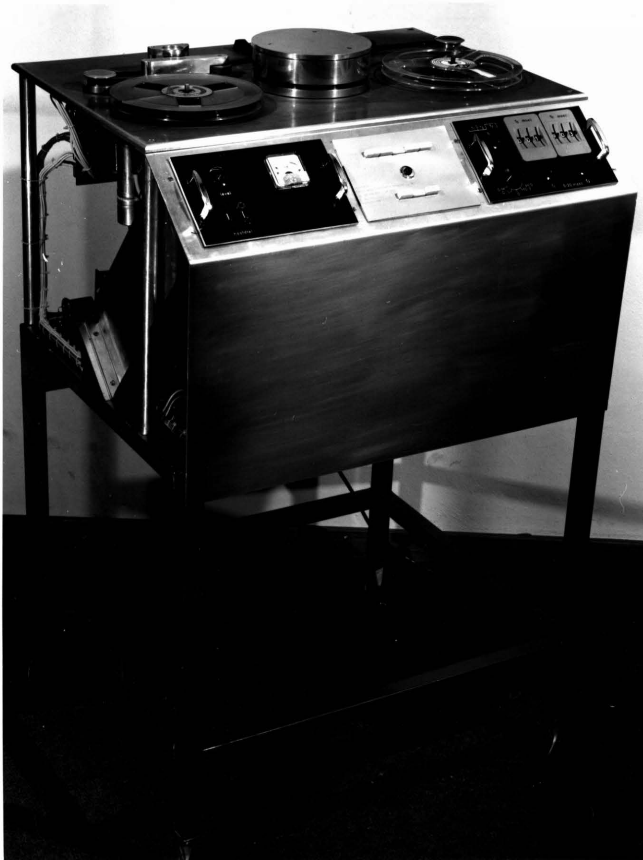
The IFA-Gate 1973 with cover removed. The plug-in unit at the right shows thumb switches for setting the width and the location of the gated interval. The plug-in unit at the left houses the output (based on peak value) amplifier with overload control. The middle section contains all switches for the transport of the tape and the manipulation of the rotating head.
