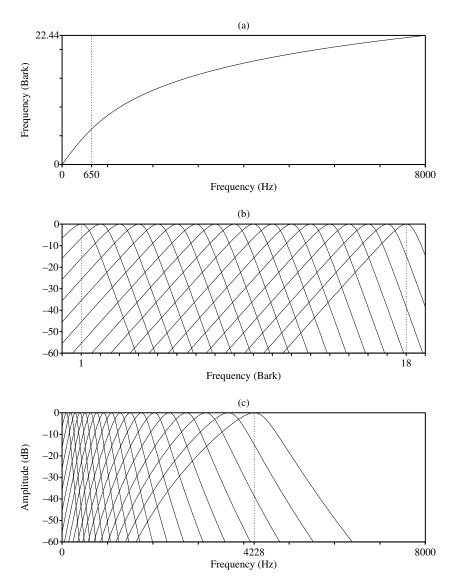
**Figure 8.6.** (a) The relation between the frequencies in Bark and Hertz. (b) The 18 filter functions on a Bark frequency scale. (c) The 18 filter functions on a frequency scale in Hertz.
