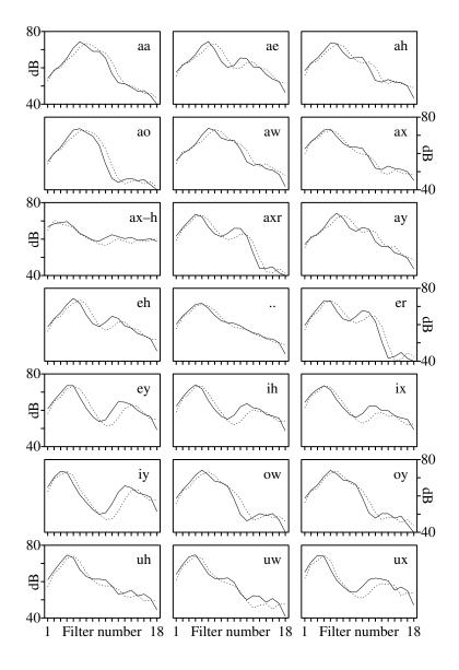
**Figure 9.2.** The average male and female vowel spectra. The male and female spectra are drawn with solid and dotted lines, respectively. The two spectra at the position in the middle, i.e. fourth row and second column, are the overall average male and average female spectra.
