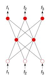
**Figure 7.4.** Topology of the supervised auto-associative feedforward neural net used for learning the associations between logarithmically scaled formant frequency values.
