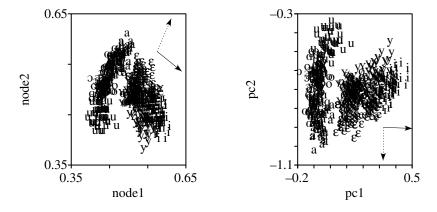
**Figure 7.6.** Two different representations of the formant frequency data scaled according to equation (7.34). Left: the representation at the hidden layer of the neural net of figure 7.1 with topology (3, 2, 3). Right: the plane with the first two principal components. The solid and dotted arrows are data taken from table 7.5 and indicate the directions of the eigenvectors for the first and second canonical correlation, respectively.
