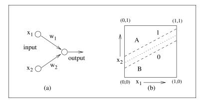
**Figure 6.1.** An example of the effect of bias change on the decision boundary. In the left figure the topology of the net is shown. The right figure shows three parallel decision boundaries  $w_1x_1 + w_2x_2 + \theta = 0$  for three different values of the bias  $\theta$  and fixed weights  $w_1$  and  $w_2$ .
