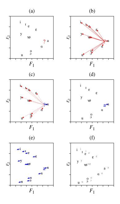
**Figure 11.1.** The adaptive vowel classifier at work. (a) An unknown vowel '?' is presented. (b) Distances are determined. (c) Find shortest distance. (d) Label as best match. (e) Move references ( $\alpha = 1$ ). (f) The new references (old references in grey).
