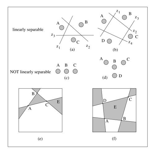
**Figure 4.2.** Linear separability in two dimensions. The elements in panels (a) and (b) are linearly separable with a one-layer net, the elements in panels (c) and (d) are not. In (e) and (f) the elements (A, B, C) and (A, B, C, D) are linearly separable. Adding a new element *E*, in the shaded area, renders the new element not linearly separable from the others.
