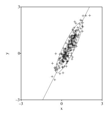
**Figure 3.1.** Bivariate normally distributed random data centered at (0.5, 0.3) in the *xy*-plane with principal direction at an angle of 60 degrees with respect to the horizontal *x*-axis. The ellipses are the  $1\sigma$  and  $2\sigma$  ellipses that include approximately 39.3% and 86.5% of the data, respectively.
