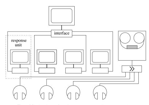
**Figure 2.3.** Listening configuration. Four response units are connected to a central unit (Apple IIe). A Revox A77 taperecorder and Sansui AU-22 amplifier provide the audio signals to the earphones.
