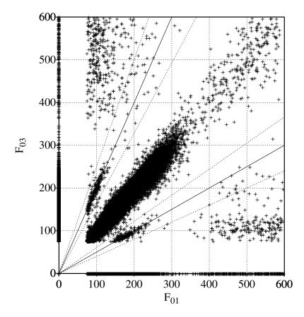
**Figure 8.5.** Scatter plot of the fundamental frequencies at the first and last position in a vowel. The two solid lines originating at the origin mark where the fundamental frequencies differ by two octaves, i.e. one octave up and one octave down from the cloud in the middle. The points on the axes mark unvoiced frames.
