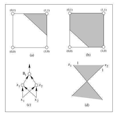
**Figure 4.3.** Graphical representation of boolean functions AND (a) and OR (b) of a neural net (c) with topology  $(A_2, B_2, B_1)$ . The XOR function cannot be made: there is no single straight line that separates both (0, 1) and (1, 0) from the other two points. In (d) the XOR-decision region in the input space is shown shaded.
