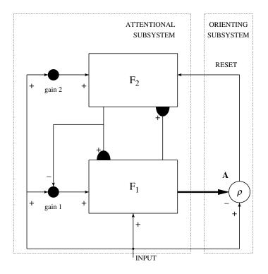
**Figure 10.2.** Typical ART neural network block diagram. After preprocessing, the input activity pattern is transformed to the first field  $F_1$ . Field  $F_1$  is connected to field  $F_2$  with feedforward and feedback connections which are indicated with black half ellipses. These connections form the long term memory components of this system.
