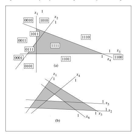
**Figure 4.4.** Two possible decision regions for two-layer nets. (a) Most simple concave decision region of net with topology  $(A_2, B_4, B_1)$ . In figure (b) the most simple hollow decision region of a net, with the topology  $(A_2, B_6, B_1)$  is shown. That side of the line where the output of the hidden node is 1 is marked.
