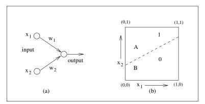
**Figure 4.1.** (a) Example of a net with topology  $(A_2, B_1)$ . (b) The dotted line separates the input space into two regions *A* and *B*.
