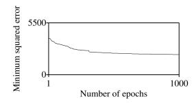
**Figure 9.9.** Typical development of the cost function during the training of a neural network with topology (9, 9, 20).
