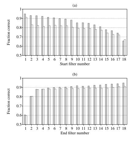
**Figure 9.5.** Discriminant classifier fraction correct as a function of filter subsets for data set MF-S (split up into independent training and test parts). The light and dark bars show the fractions correct with and without covariance matrix pooling, respectively. (a) Subset with filters from *i* to 18, where i = 1..18. (b) Subset with filters from 1 to *j*, where j = 1..18.
