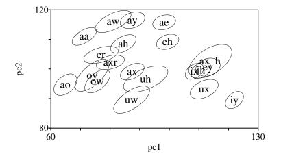
**Figure 8.8.** The positions and 0.5  $\sigma$  ellipses of the 20 vowels in the principal component plane as averaged over the 326 male speakers in the training part of the TIMIT database. The horizontal axis was inverted to get the main axes of the ellipses to point from the lower left to the upper right. The first and second principal components explain 52% and 16% of the variance, respectively.
