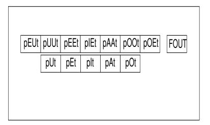
Figure 2.4. Layout of the keybord part of the response unit.
