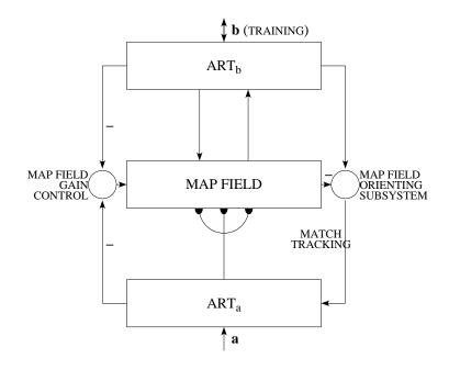
**Figure 10.1.** Block diagram of a supervised ARTMAP system. Two ART modules are linked by an inter-ART module called the map field. The map field forms predictive associations between categories of the ART modules and realizes a match-tracking rule. If  $ART_a$  and  $ART_b$  were disconnected each module would self-organize category groupings for their respective input sets.
