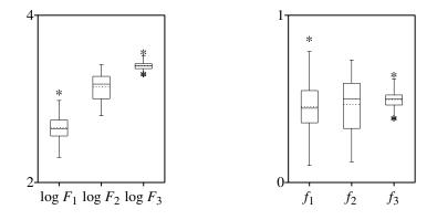
**Figure 7.5.** Box plots before (left) and after (right) scaling the logarithmically transformed frequency values. The  $f_i$  are scaled to the interval (0, 1) according to equation (7.34). The dotted lines in the box plots indicate the mean values.
