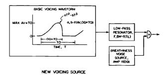
FIG. 10. Block diagram of the voicing source for the KLSYN88 formant synthesizer. The effects of the radiation characteristic have also been folded into the source models, resulting in a voicing source spectral output (Fig. 11) that falls off at about 6 dB/oct [corresponding to  $U'_g(t)$ ] and an aspiration source spectrum that is essentially flat over the frequency range of interest.
