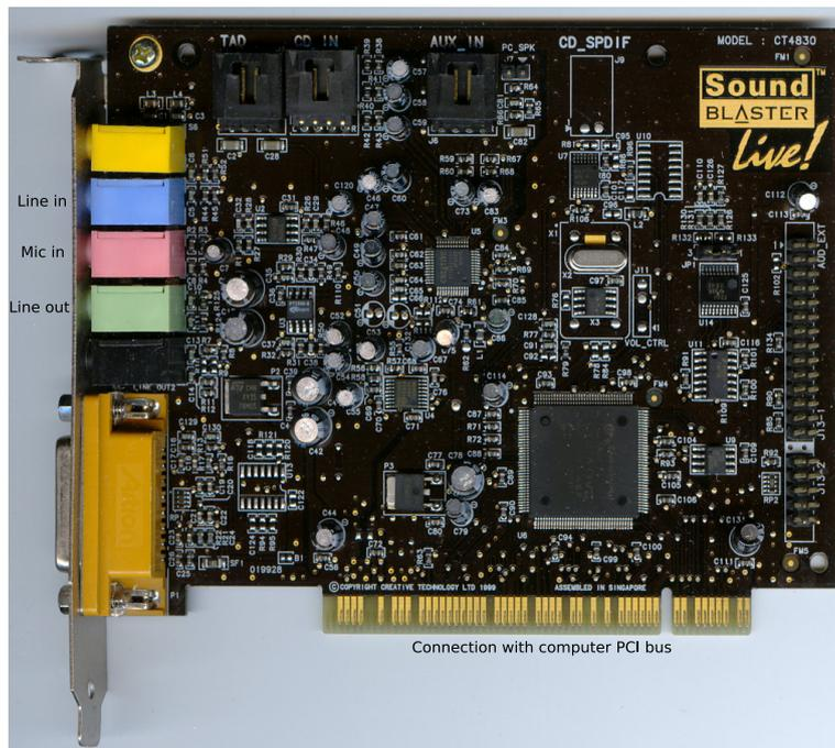
**Figure 3.3.:** A typical sound card.
