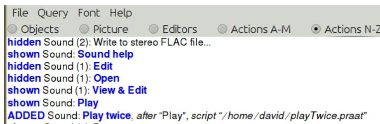
**Figure 4.4.:** Part of the buttons editor after first choosing “Actions N-Z” followed by scrolling to the actions for a Sound object.
