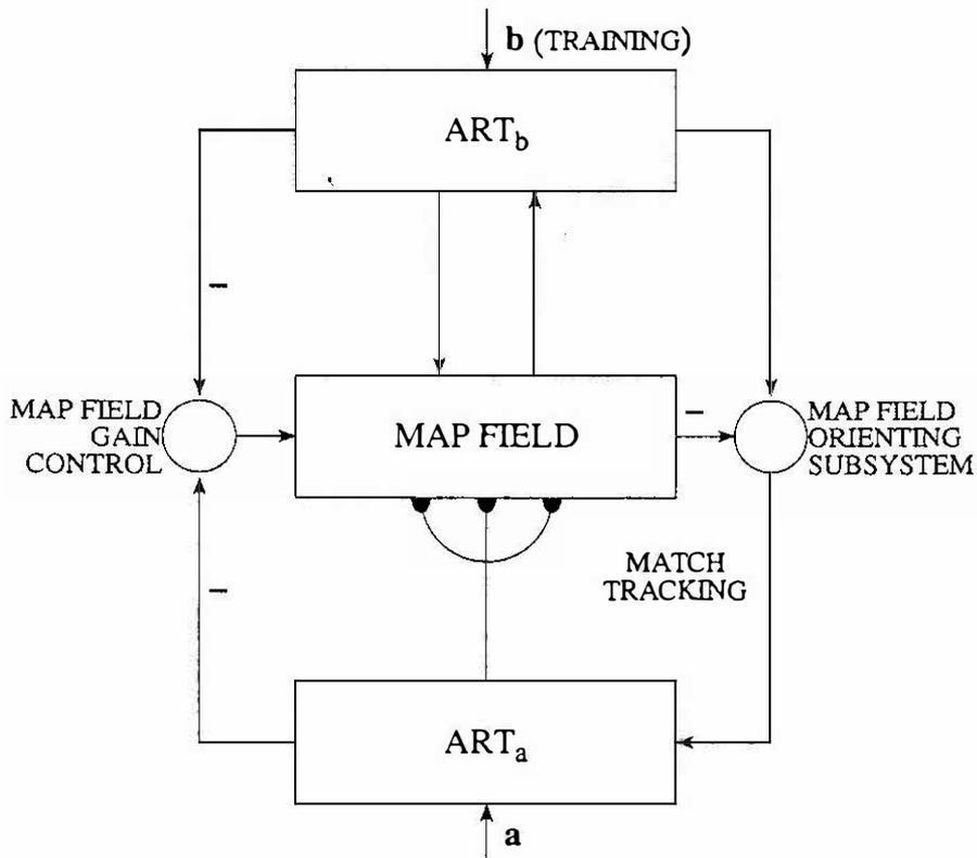
Fig. 1. Block diagram of a supervised ARTMAP system. Two ART modules are linked by an inter-ART module called the map field. The map field forms predictive associations between categories of the ART modules and realizes a match tracking rule. If  $ART_a$  and  $ART_b$  were disconnected each module would self-organize category groupings for their respective input sets.
