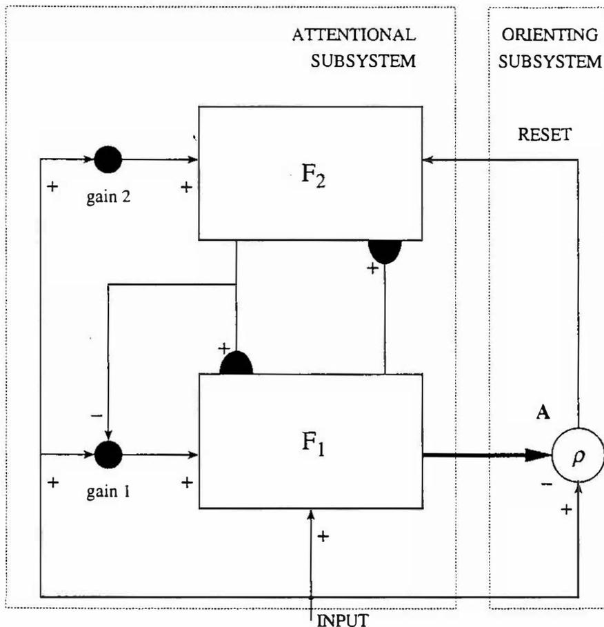
Figure 2. Typical ART neural network block diagram. After preprocessing, the input activity pattern is transformed to the first field  $F_1$ . Field  $F_1$  is connected to field  $F_2$  with feedforward and feedback connections which are indicated with black half ellipses. These connections form the long term memory components of this system.
