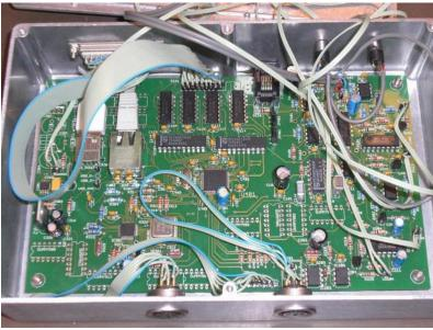
Figure 5: EventBox with internal electronics
